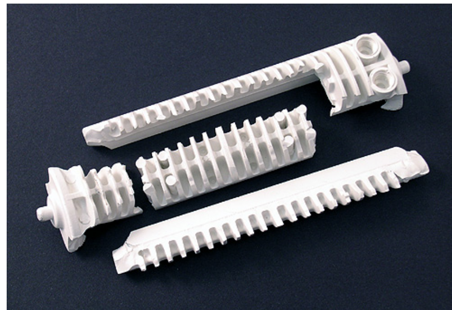
Fig. 15 – radiators broken during extraction
