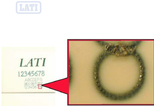
Fig. 15 LASULF white (PSU): darkening + slight foaming effect
