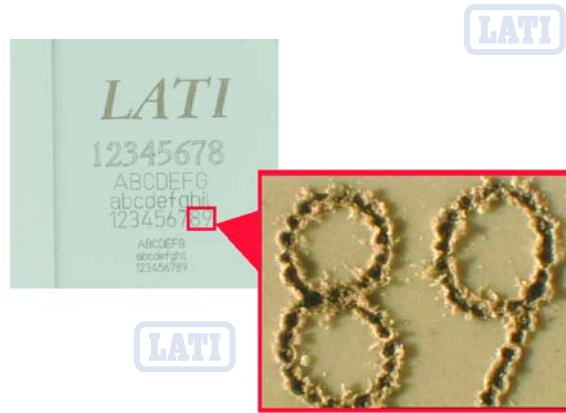
Fig. 14 KELON B FR H2 CET/30-V0 (PA6, mineral filled, FR with halogens): engraving + colour change. Visible engraved points at low magnification. At a normal distance the marking appears good readable.
